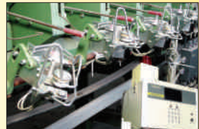
Electronic Yarn cleaner system at TIFAC Core in Textile Technology and Machinery, Kumaraguru College of Technology, Coimbatore
