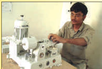
Friction Tester facility at TIFAC CORE in Industrial Safety, Mepco Schlenk College, Sivakasi
