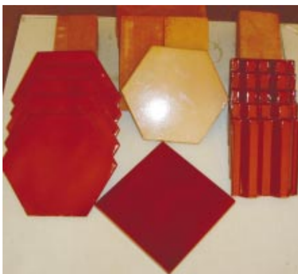
Products Developed Using 80% Fly Ash Through Firing Process Implemented by RRL Trivandrum
